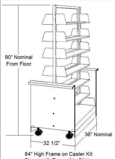
84" High Frame on Caster Kit Shown with Reversible Skirt in down position with Flat Base and Adjustable Shelves
