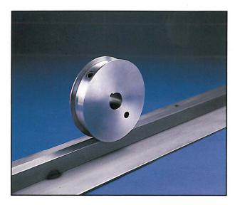
Heavy steel track bar is welded to 6" wide, 11 gauge track plate. 5" wheels, precision ground and angle flanged on both sides, ride smoothly on the track assembly.
