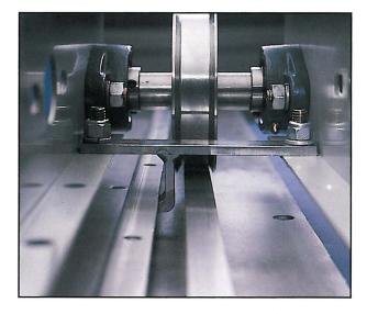
Track, "Z" bracket and trim plate are overlapped, staggered and layered construction for increased strength. A welded solid 1/4" steel bar, anti-tip "J" bracket rides within the 11 gauge "Z" bracket providing stability and meeting the strictest seismic requirements.
