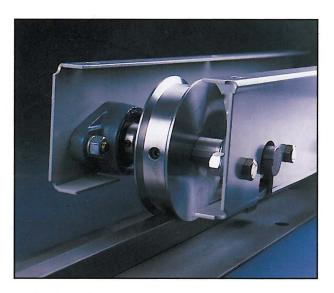
Mobile carriages are fitted with a 1" full length solid steel drive shaft connecting all drive wheels. Shafts are contained within self-aligning, flanged pillow blocks with permanently sealed and shielded bearings.
